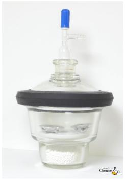
Additionally, solid material can be dried on watch glasses in drying cabinets or dessicators.
